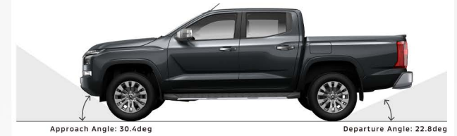
Approach Angle and Departure Angle
